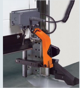
The non-contact, automatic safety cut-out protects people and property
