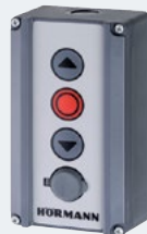
Push button DTH RM For separate control of both operational directions, with separate stop button. With miniature lock: Operator is deactivated. It is not possible to move the operator (2 keys included in the scope of delivery). Protection category: IP 65 Dimensions: 90 x 160 x 55 mm (W x H x D)
