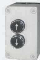
2-key push button For separate control of both operational directions. Protection category: IP 44 Dimensions: 70 x 118 x 65 mm (W x H x D)
