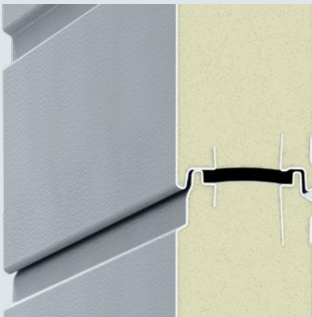
Sections with thermal break in SPU 67 Thermo
