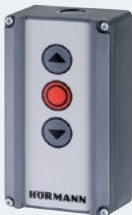
Push button DTH R For separate control of both operational directions, with separate stop button. Protection category: IP 65 Dimensions: 90 x 160 x 55 mm (W x H x D)
